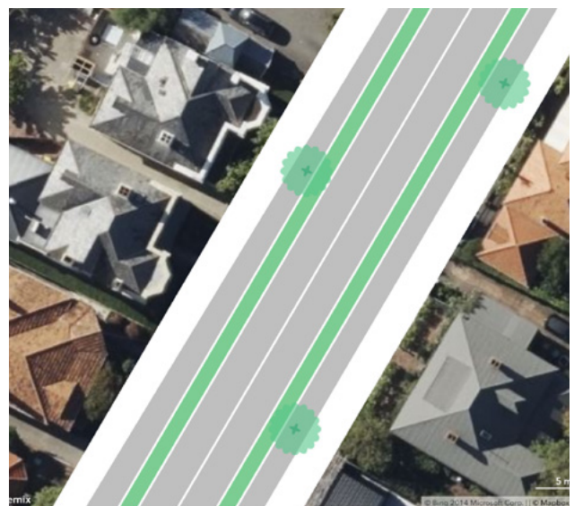
Top and Centre: De Witt Street existing conditions Bottom: De Witt Street with proposed buffered bike lanes
